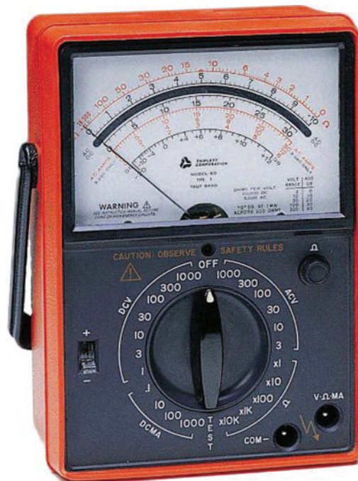
FIGURE 9-6 Volt-ohm-milliamperemeter with multirange selection. Courtesy of Triplet Corporation
