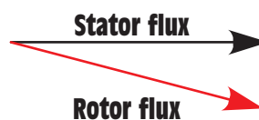
FIGURE 32–32 Rotor and stator flux become more in phase with each other as motor speed increases.
