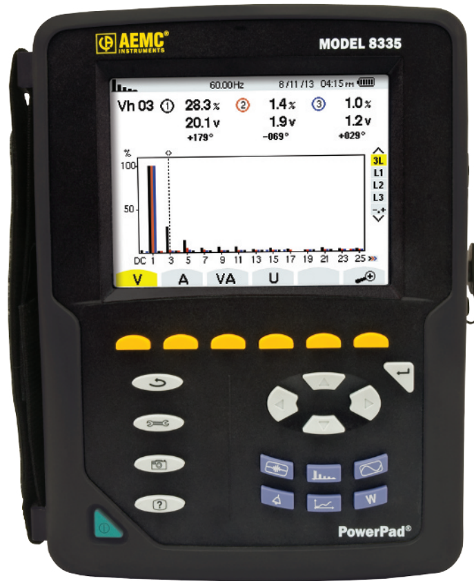
FIGURE 35-9 Power meter with harmonic display. Courtesy of AEMC® Instruments
