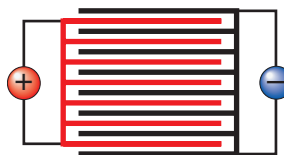
FIGURE 12-22 Multiple plates increase the surface area and the amount of current the cell can produce.
