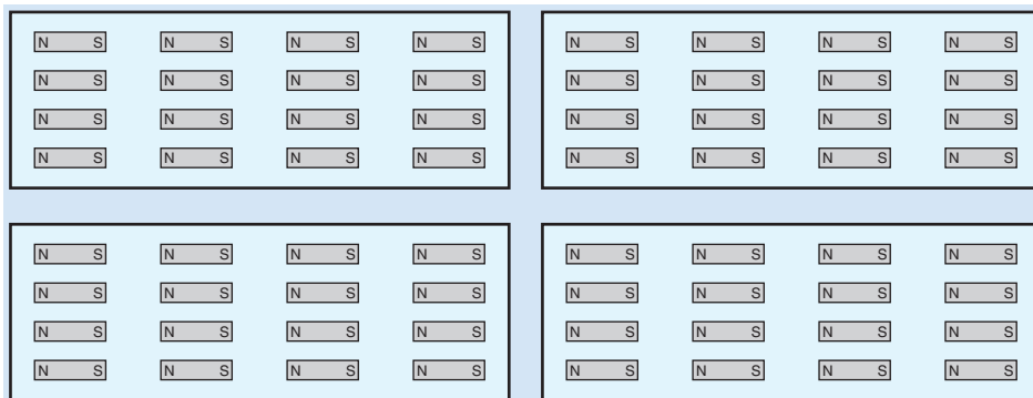
FIGURE 4-7 When a magnet is cut apart, each piece becomes a separate magnet.
