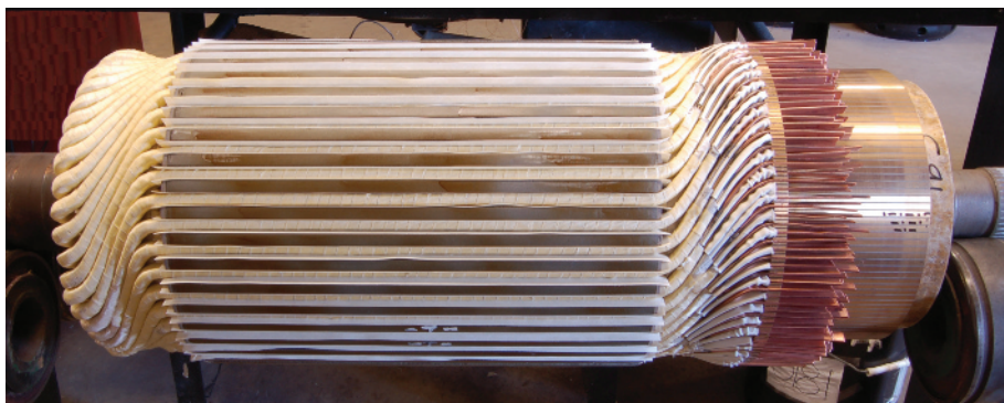
FIGURE 29-24 Armature wound with rectangular wire. H.L. Hailey Enterprises, Inc. - Longview, TX
