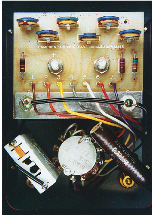
FIGURE 9–23 DC ammeter with an Ayrton shunt.
