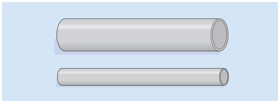
FIGURE 10-14 A large pipe has less resistance to the flow of water than a small pipe.
