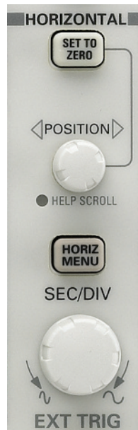
FIGURE 9-53 Time base control for a typical digital oscilloscope. Courtesy of Tektronix, Inc.
