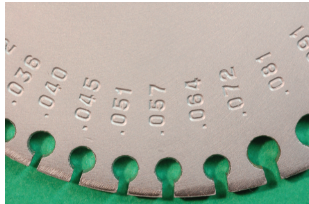
FIGURE 10-4 The other side of the wire gauge lists the diameter of the wire in thousandths of an inch.
