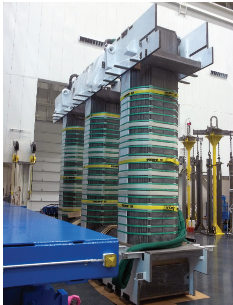
FIGURE 27-28 Core of a 630-MVA three-phase transformer. Courtesy of SPX Transformer Solutions, Inc.
