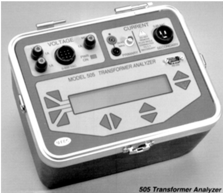
Figure 11-36. Instrument for Measuring Current Transformer Secondary Admittance and Burden.
