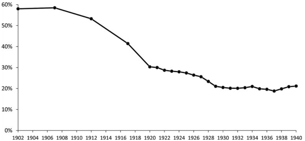
FIGURE 2.3. Proportion of electricity made available in the United States from nonutility sources
