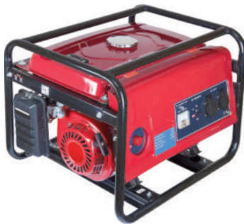
FIG. 20.43 Single-phase portable generator. (Yevgeniy11/Fotolia)
