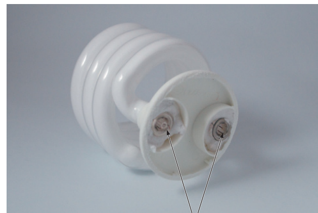
Connections to electronic ignition network
