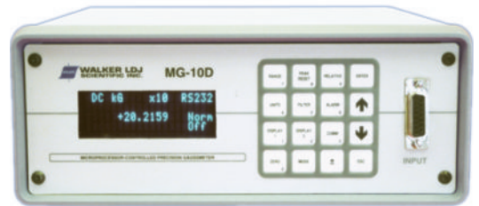
FIG. 11.14 Digital display gaussmeter. (Courtesy of Walker LDJ Scientific Inc. www.walkerldjscientific.com )
